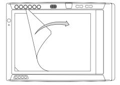
Figure 3-3 Removing the protective cover
